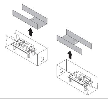
Step #3: Replace wiring compartment covers.
