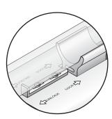
C. With the lamp properly installed, the clip is moved into its final locked position.
